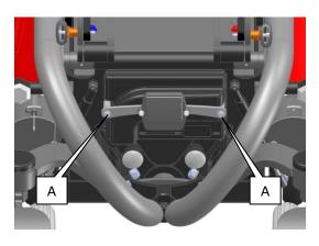
Remove the back cover in the middle first (see chapter 8.1.). Unscrew the screws (A), and then you can tip the power module back. Unplug all plugs from the power module. Switch the power module and plug in the plugs again. Mount the new power module on the wheelchair with the two screws.
