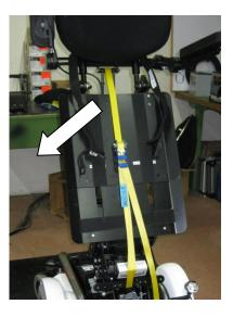
Hold the seat to release the tight down system and let it down slowly towards the neutral respectively the non-tension position
