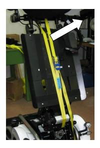
Pull the seat in most standing position to enforce the actuator unit
