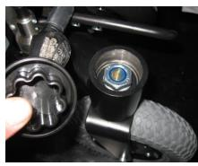
Remove the cover cap by pushing upwards. Unscrew the nut until it could be taken out.
