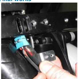
Positioning and adjustment of the speed limit switch.
