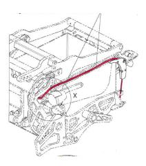
The routing is above the light and indicator support. The deviation starts from this point.
