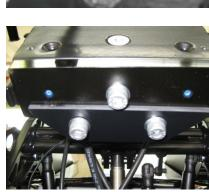
The screws has to be positioned. But only tighten it when every screw is placed.
