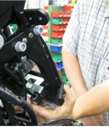
Place the actuator support into the leg rest assembly.
