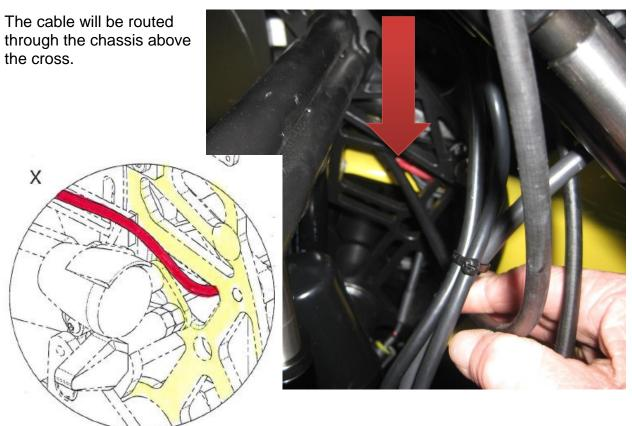
The left cable will be overcrossed to the right cable and fitted to the actuator unit respectively attached at the levers of the Rosta element.
