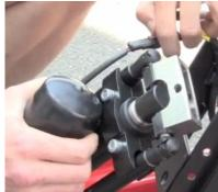
Plug in the Actuator unit at the control and move it in as short as possible
