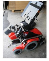
**CAUTION** – Before working on the standing actuator, the chair has to be brought into a full standing and tilted position to release the system.
