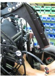
The actuator is now fully released and can be taken off from underneath the leg rest assembly including the gas cylinders. Some turning movement would help feed out it easy.
