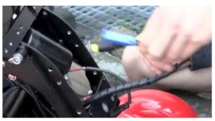
Now the cables will be feed from the front to the rear between the gas-cylinder and the actuator.
