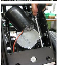
If the support is positioned properly, tighten as first the base plate and then counter sunk screw and after the allen screws.
