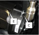
Now pull the cables from the other end (C) through the magnetic brake levers on the motor top end.
