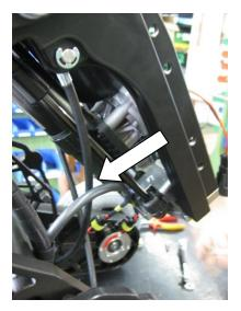
Push the actuator unit towards the lowering cables. Take a tool to feed it to protect your hand and fingers!
