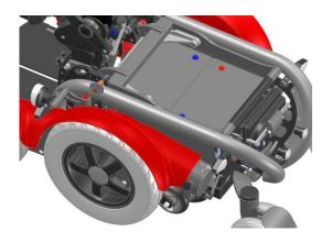
Raise the wheelchair into the standing position and remove the middle cover in the back (see chapter 8.1.). Push the pole cover back and unscrew the screws on the battery poles.
