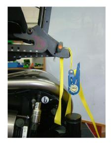
If the standing actuator is unscrewed, release the tight down system slowly and carefully.
