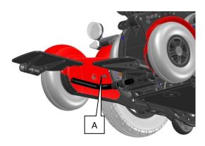
Unscrew the screw (A) below the foot plate, now you can remove the foot plate from the tube. Mount the new foot plate and put the screw back in place and tighten it.
