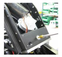
Unscrew the two allen screws of the base plate inside the leg rest assembly.
