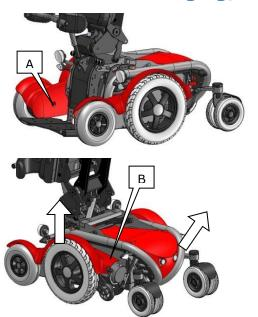
The covers are attached with screws, clips and velcro.
