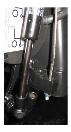
Adjusting the length of the shock absorber (A) will allow a fine tuning of the front wheel to the floor clearance as well as the suspension of the chair. Make sure the chair is in seating position.
