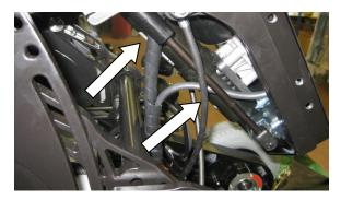
The cable has to be routed from behind between the lowering cables and gas-spring and actuator towards the front (at least to the rear) respectively the actuator plug.
