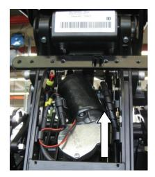
Now the actuator unit raise up towards the cable supports. If necessary, feed the actuator slowly towards the neutral respectively the non-tension position. Take a tool to feed it to protect your fingers!
