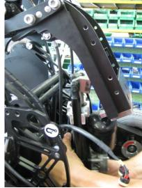
The stand up actuator unit can be taken off from underneath the leg rest assembly. Assure that the front wheel cables are behind the unit.
