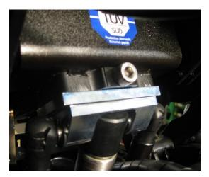
Loose the coupling bolt at the base underneath the seat so that it could be unscrewed later by hand.
