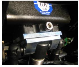
Move your position to the left or right side of the chair to hold the actuator in one hand and to unscrew completely the coupling bolt underneath the seat.
