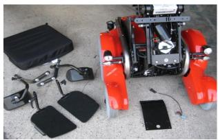
The speed limit switch has to be disassembled and unplugged.
