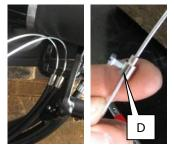
Enter the new cables the other way around and mount the brake release lever again. Now bring the cylinder head (D) to the position closely to the brake release lever where the cables are getting through and fasten the clasp screw (A) of the cylinder head (D) again.
