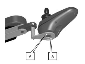
Remove all cable cords from the joystick cable all the way down to the seat pan and unthread the cable. Unscrew both screws (A) under the joystick, now you can replace the joystick module.
