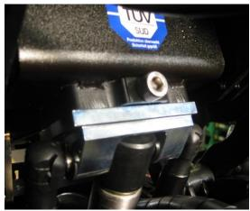
Move your position to the left or right side of the chair to hold the actuator in one hand and set the coupling into the coupling base underneath the seat.
