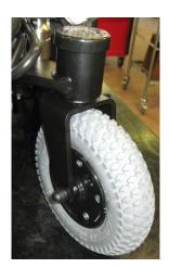
Remove the cover cap in the middle of the **7" twin wheel** by using a fine screw driver to lift the cover cap off, do that with both wheels. Unscrew the screw going through both wheels and now remove the worn wheel. Now mount all pieces back together, the other way round.
