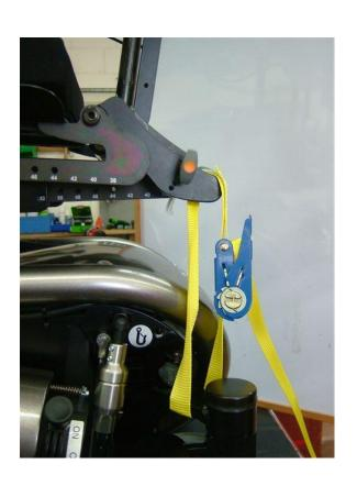
If the chair is in seating position, assure the seat is secured by a tightening system to not go up. But it has not to be tight down more than the position is given by the actuator. Otherwise the assembling
