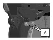
Unscrew the 4 screws (A), and then slide the seat back or forth. When you reach the required position, put the screws back in and tighten them again.
