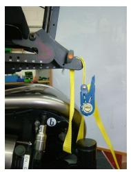
CAUTION - The seating system is tension loaded for standing configuration and is held back by the standing actuator. Before loosening the standing actuator, assure the seat is secured by a tightening system.
