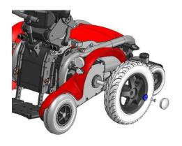
Bring the chair into the standing position to lift the middle wheels off the ground.
