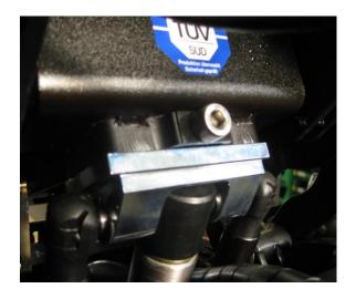
Move your position to the left or right side of the chair to hold the actuator in one hand and to unscrew completely the coupling bolt underneath the seat.
